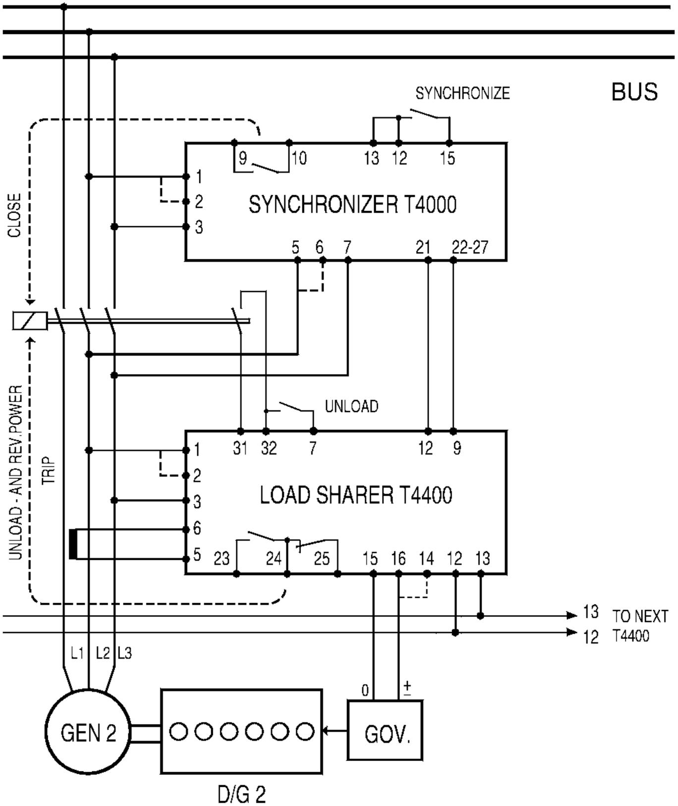
1000, T4400 and speed controller with -5V to +5V DC input.
